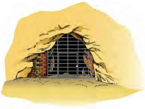
Fig. 12.6. The cave entrance is closed with a grille. On the left, bars are strengthened to support the wall. On the right, they are embedded directly into the wall. The grille has a door with a lock. Drawing by D. Segliņa.
