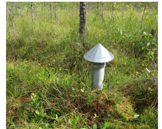
Fig. 9.3. A bore-hole for monitoring of water level in Veseta floodplain mire. Photo: A. Priede.
