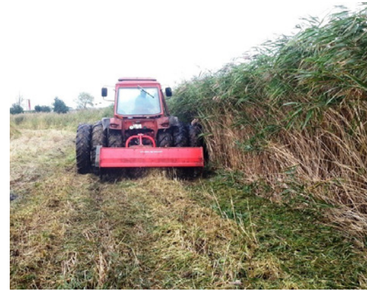
Fig. 15.45. Triple-wheeled tractor can be used for mowing in wet meadows and alkaline fens overgrown with reeds. The photo is taken in a heavily overgrown floodplain meadow in Latvia with similar conditions as in overgrown fens. Photo: A. Liepa.
