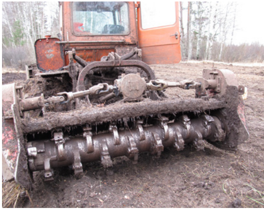
Fig. 15.41. A crawler tractor equipped with a mulcher. Photo: A. Liepa.
