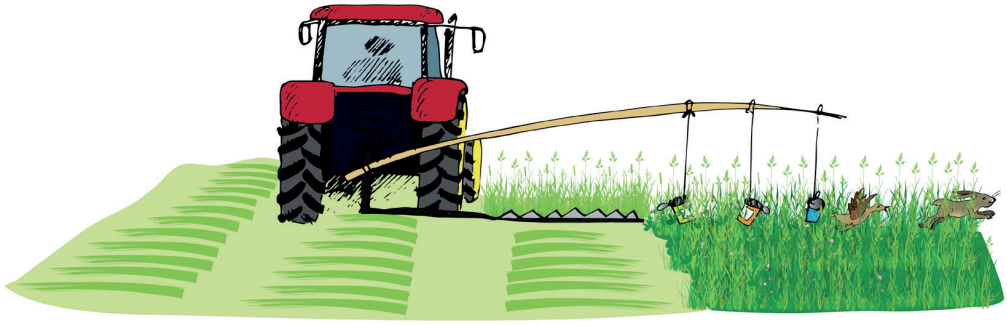
Fig. 22.2.9. Cans filled with stones are fixed to a long pole. Cans are situated above the grass strip that will be mowed next (next to the mower) (Kronitis 1982). Drawing by D. Segliņa.
