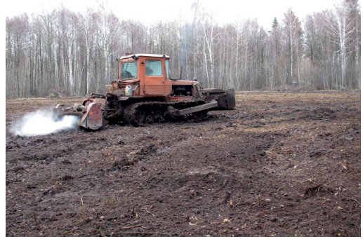
Fig. 15.5.2. Grinding of grassland in Čaukciems meadows in Ķemeri National Park in January 2013. Shrubs and separate trees were cleared and removed before grinding, except for older tree clusters and some individual trees. In grinding, "islets" of vegetation around tree clusters were left. Grinding was done in the snow-free period when the ground was not frozen. Photo: A. Liepa.
