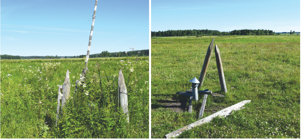
Fig. 7.4.7. The groundwater table monitoring wells and surface water level measuring stakes must be surveyed and restored each year, especially in areas where floods occur or grazing animals are used. Condition of wells and stakes in 2015 constructed in Dviete floodplain in 2012. Photo: S. Rūsiņa.
