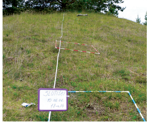
Fig. 7.4.3. Arrangement of sample plots in a transect with spacing of 2 metres. The transect starting point is fixed at the pine, where a 30 cm stake is driven into the ground. It is located each year using a GPS receiver and metal detector. The direction of the transect is determined by measuring the azimuth with a compass and sample plots are established with an interval of 2 metres, marking the first sample plot two metres from the transect starting point (to prevent the impact of trampling on vegetation during the localisation of the transect). Photo: S. Rüşîa.
