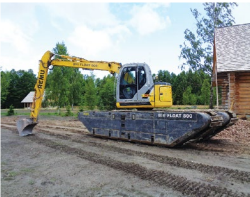
Fig. 13.6. Floatable machinery Big Float for reopening of water circulation and fish migration channels in dense mineralised reed masses. L. Engure. Photo: J. Reihmanis.
