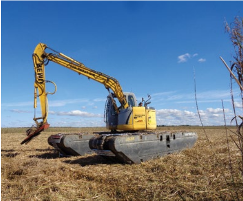
Fig. 13.5. Fragmentation of reed stands with a specialised cutter in Lake Engure. Photo: J. Reihmanis.
