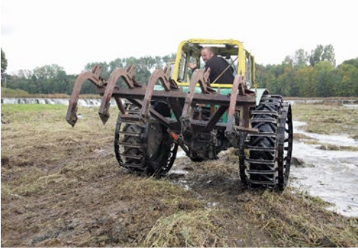
Wheel tractors equipped with metallic chains for better stability. R. Venta. Photo: A. Lācis.
