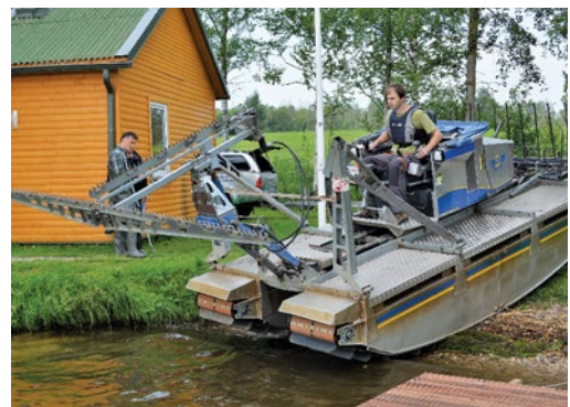
Floatable TRUXOR equipped for mowing of macrophytes suitable for management of larger areas. Rāzna. Photo: Ē. Kļaviņa.
