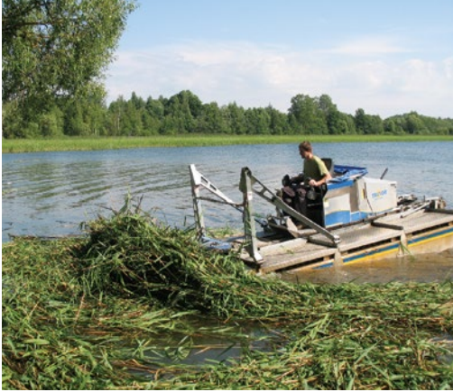
Fig. 13.10. Removal of cut reeds with TRUXOR equipped with a specialised rake.
