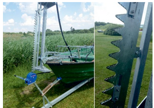
Fig. 17.27. Macrophyte cutter mounted to a boat. Suitable for deeper rivers and lakes. Photo: L. Urtāne.
