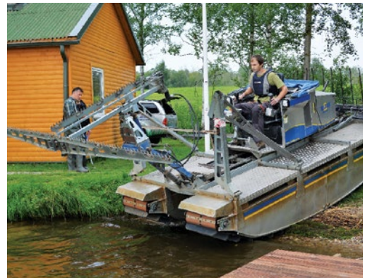
Fig. 13.7. Floatable machinery can be equipped with reed cutter, an excavator, sediment sucking equipment as well other tools facilitating diverse activities. Photo: Ē. Kļaviņa.
