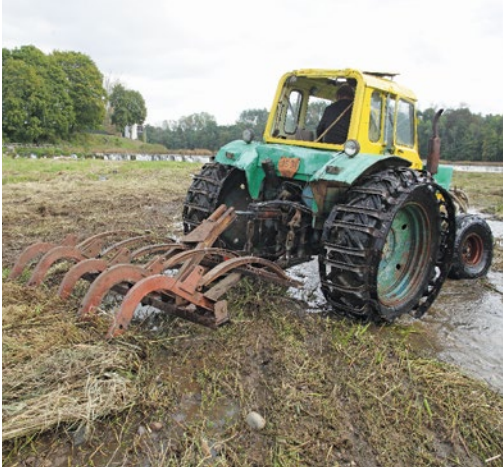
Fig. 17.28. In the River Venta, a wheeled tractor is used in order to reduce the aquatic plant overgrowth and to scarify the root system. To provide additional grip, the tractor is equipped with metallic wheel wrappers. Photo: A. Lācis.
