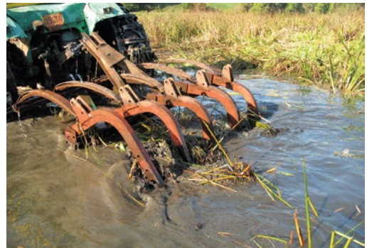
Harrows for shearing of the root system in action. R. Venta. Photo: A. Lācis.
