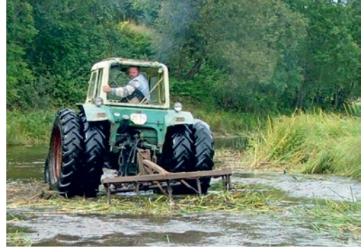
For stability, a double wheel system can be used. R. Salaca. Photo: A. V. Urtāns.
