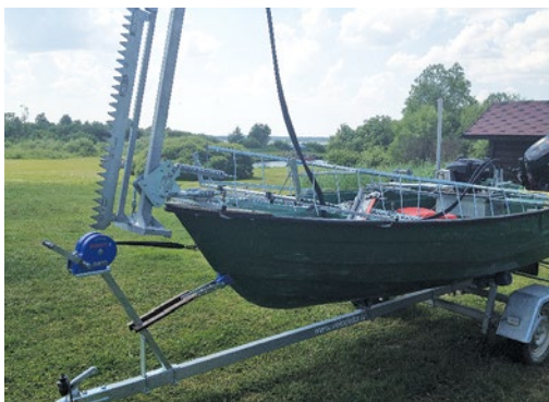
Macrophyte cutter mounted on a boat suitable for mowing of larger areas. L. Durbe. Photo: L. Urtāne.
