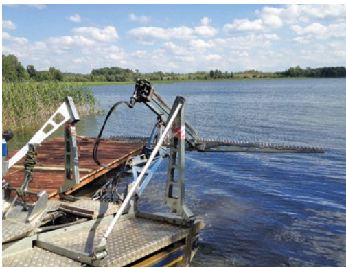
Fig. 13.8. Floatable TRUXDR equipped for mowing of macrophytes suitable for management of larger areas. Photo: L. Urtāne.
