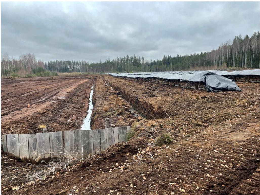
Figure 2. Example of block-cutting in the western part of the Unguri peat production area (STEIGER Engineering, 08.11.2022)
